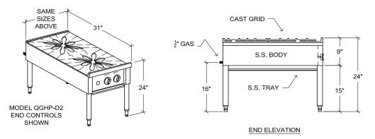
APPROVED FOR INSTALLATION ON COMBUSTIBLE SURFACE WITH A MINIMUM CLEARANCE OF 12" TO THE SIDES AND 18" TO BACK FROM ADJACENT COMBUSTIBLE WALLS. OPTIONAL HEIGHT UP TO 36"
